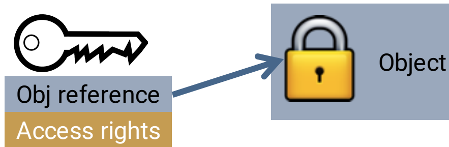
Figure 2.10: A capability is a unique token which contains specific rights to a particular object. Figure source [1].
